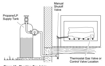
Figure 16 - Checking Gas Joints
